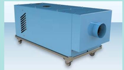
This additional kit can be mounted to the back of the noise reduction box. It allows to connect the noise reduction box to the lab exhaust system so the waste heat of the pump gets out of the lab. If the lab exhaust system should fail, the exhaust is not blocked but blows into the lab to ensure the cooling of the pump.
